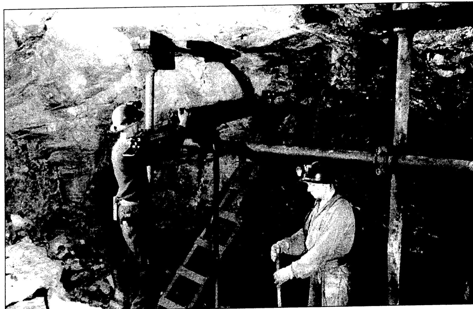
Miners with their drill set up in a stope undercut in this photo taken at the mine in 1947.
